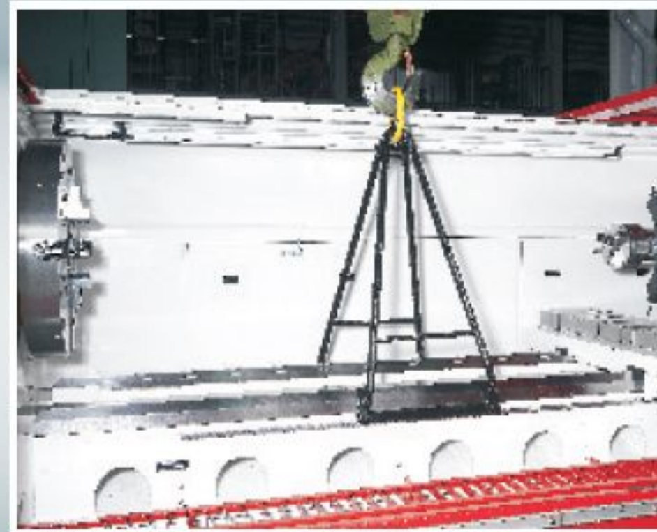
RIC-TC43 / 52 / 62 series CRANE LIFTING DEVICE (STD.)
