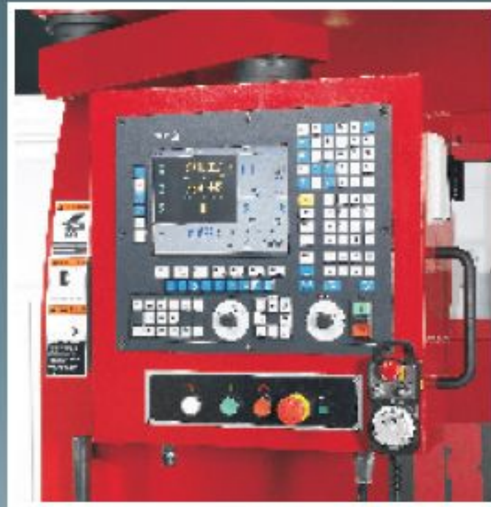
RIC-TC43 / 52 / 62 series CONTROL PANEL + MPG WITH EMERGENCY STOP BUTTON (OPT.)
