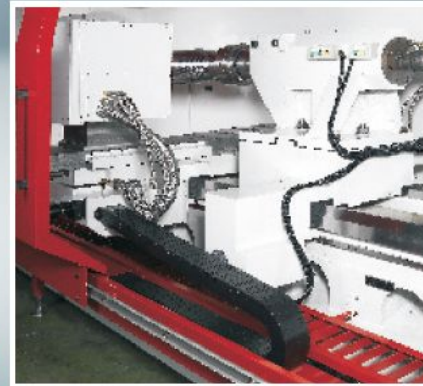
RIC-TC43 / 52 / 62 series TAILSTOCK WITH A1-8 SPINDLE + 10" 3-JAW STRONG CHUCK (OPT.)
