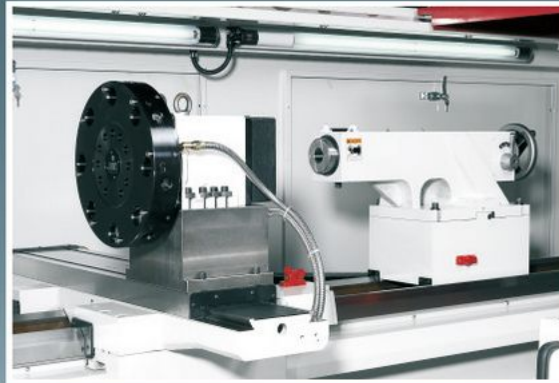
RIC-TC33120 WITH SAUTER 8 POSITION ELECTRICAL TURRET + VDI 40 (OPT.)
